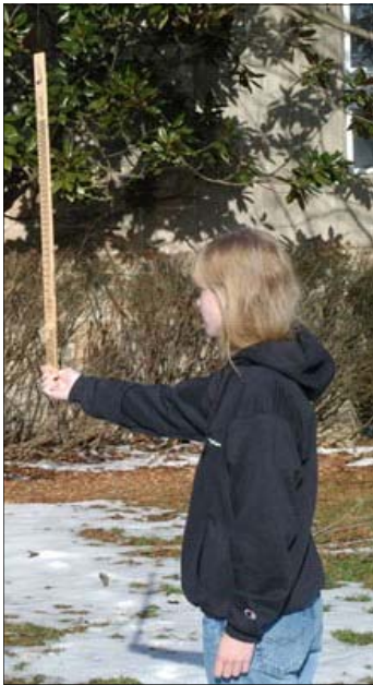
Measuring tree height – Biltmore or Tree Scale Stick
