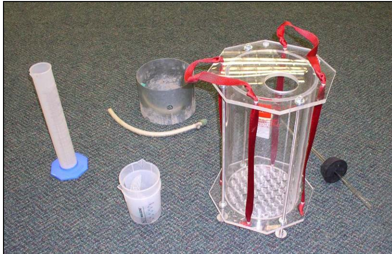
Figure 4.2. Infiltration Equipment (Left to Right): Graduated cylinder, overflow collection tubs, overflow tube, metal ring, and infiltrimeter.
